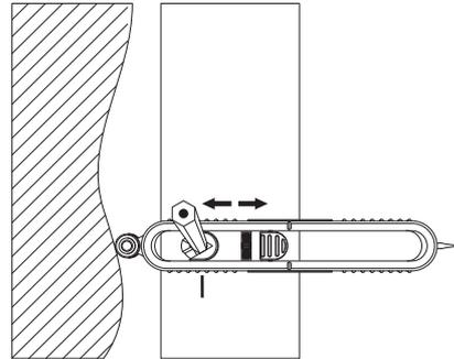
With the wheels in contact with the wall, set the distance by moving the pencil holder to align the pencil point with the mark.
