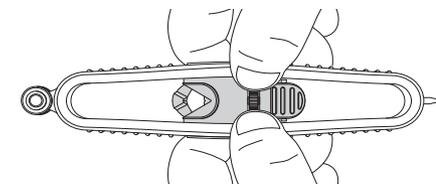
The pencil holder can be removed and rotated to face the opposite direction to bring the pencil closer to the easy glide tip.
