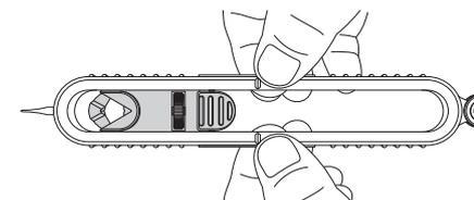
Pull the loop apart to reinsert the Pencil Holder in the opposite direction as shown.
