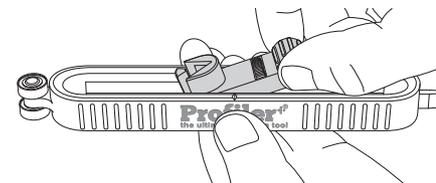
With pencil holder in the centre, grip the loop and pull apart, push the pencil holder out.
