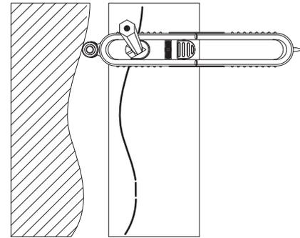
Steadily move the Profiler+® perpendicular to the wall along the entire length of your material to reproduce the outline of the wall.
