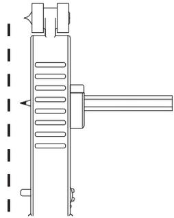
For best results, insert the pencil or other marking implement through the holder as shown, align with prongs and tighten securely.
