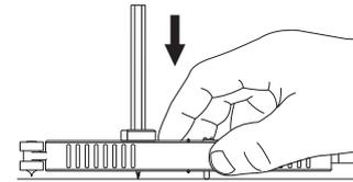
Apply a gentle pressure between the pencil and thumb wheel so that the two prongs and pencil tip remain in contact with the material to stabilise the Profiler+® during scribing.
