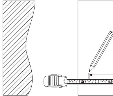
Measuring towards the edge of the material to be scribed, put a mark indicating the width or length of material that needs to remain after cutting.
