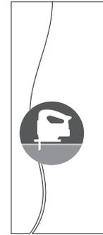
Cut along the line, leaving the pencil line showing on the piece you require. This allows fine adjustment after cutting still having your pencil line to work to.
